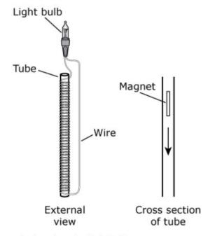
When the magnet is falling through the tube, the light bulb turns on.
