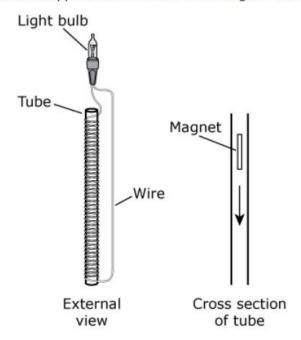
When the magnet is falling through the tube, the light bulb turns on.
